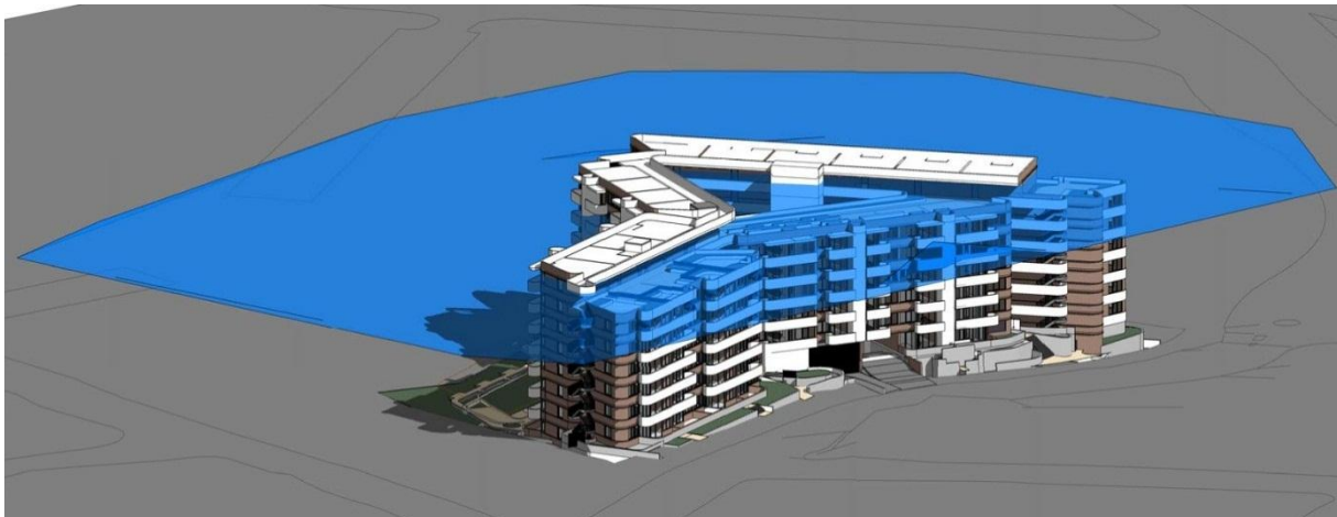
Figure 7: Diagram of height of building non-compliance resultant from flood planning level shown above the blue plane.
